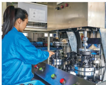
控制阀扭矩定值装配设备 Fixed torque assembly machine for control valve
